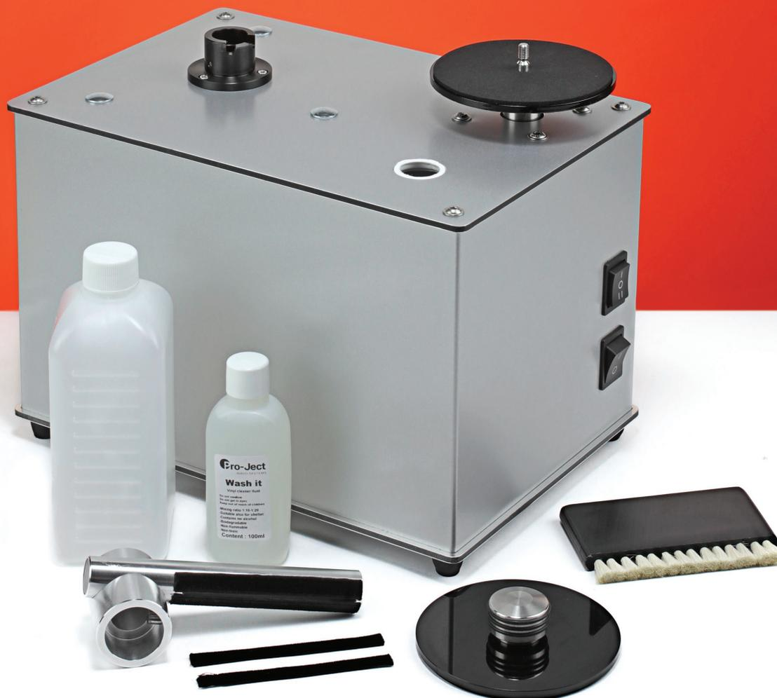
*On top of the main unit you can see the pivot for the suction arm, the lower disc-clamp and the reservoir drain hole. Arranged around the base are the upper clamp, the arm (with spare velvet pads) and the brush that's used to spread diluted cleaning fluid over the record. The latter is prepared by mixing concentrate from the smaller bottle with tap water in the larger one - embossed with horizontal lines to help ensure correct proportions.*
